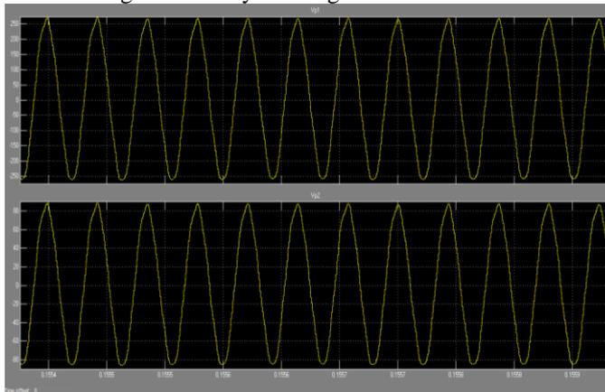
**Fig 12: Waveforms of Voltages across primary winding 1 and 2 which shows load resonant frequency is twice the switching frequency**
