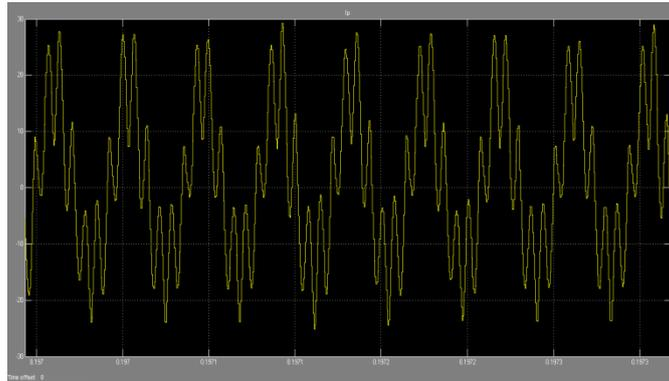
**Fig 11: Primary winding current waveform**
