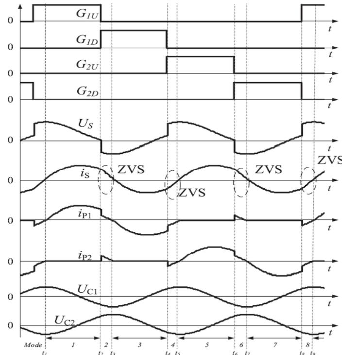
Fig 3: Operating waveforms of proposed inverter
