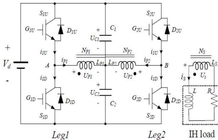
Fig 2: Simplified schematic diagram of multiple frequency resonant inverter
